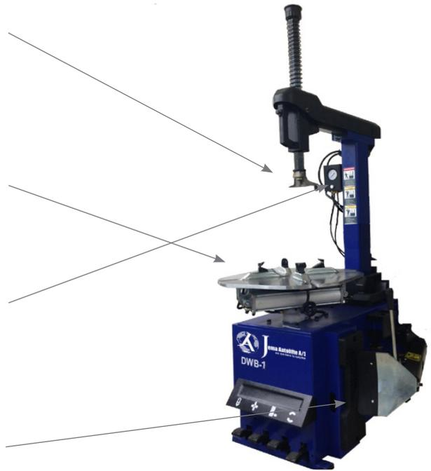
DWB-1 is Full automatic pneumatic tilting column, pneumatic locked at optional position. Powerfull air booster makes the tyre and rim jointed instantly. DWB-1 is suitable for low profile tyres. The tyre changer DWB-1 is CE approved
